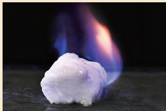
▲ Gas hydrates easily catch fire as methane gas is emitted in high-temperature and low-pressure environments.
