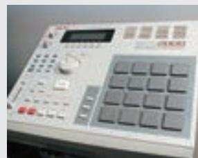
▲ The sampler uses sound recordings(or samples) of real instrument and these samples are usually stored in digital memory.
