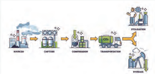
▲ CCUS goes through three stages: (1) capture, (2) compression and transportation, (3) storage or utilization.
