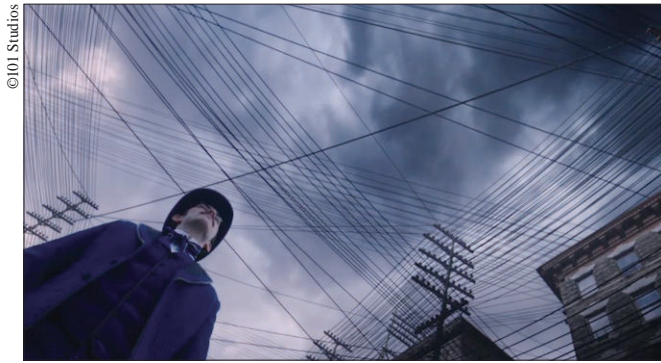
▲ Westinghouse realizes that too many powerlines are needed when using DC generators.
