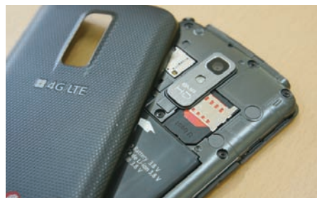
▲ USIM is located at the back of phones. It could be replaced to another USIM.
